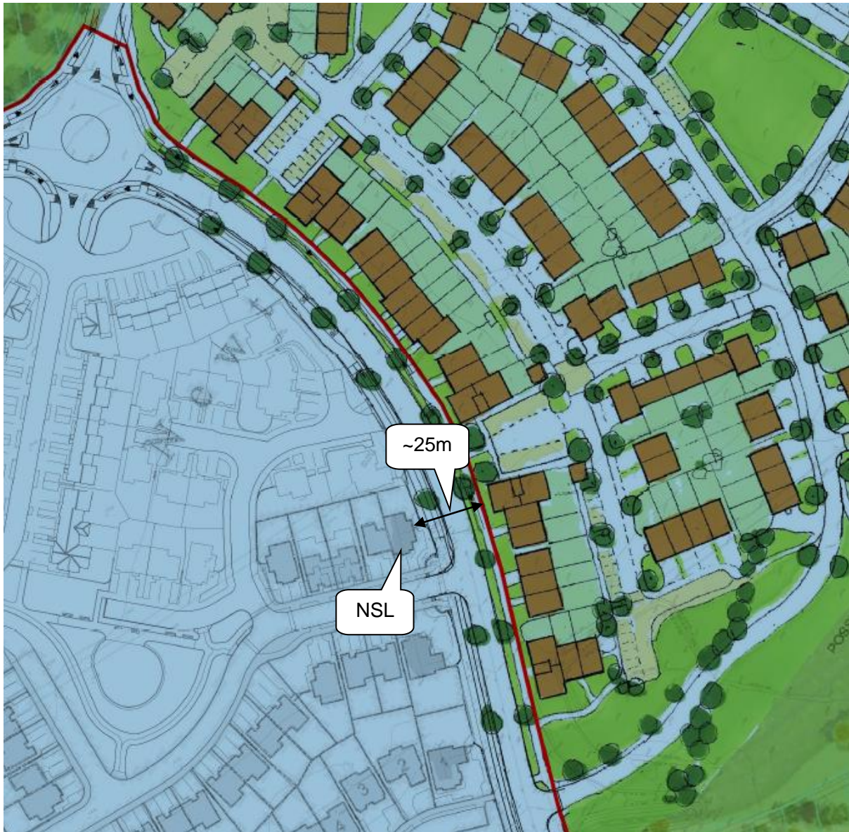
Figure 11-5 Representative Noise-sensitive Location (NSL)
