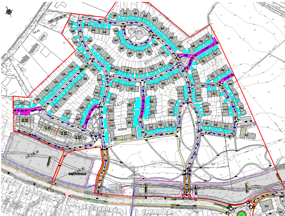
FIGURE 9-9 PROPOSED OVERLAND FLOW ROUTE (NORTH SITE)
